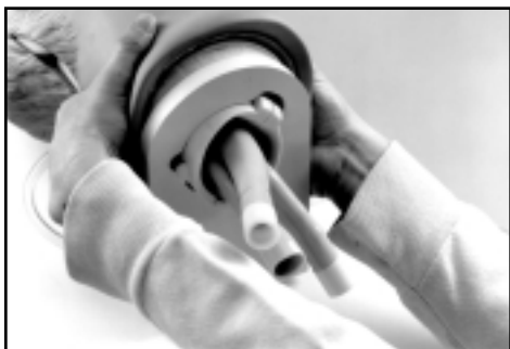
Figure 4 Next, turn the head slightly to the side to align the keyways with the slots, and pull the head from the stand (Figure 4).
