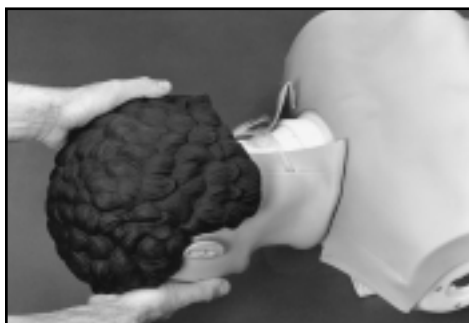
Figure 5 Next turn the head face down and begin inserting it at the shoulders. Tip the head upward slightly until the two keyways on the rear of the neck slide under the ring and into the top of the torso (Figure 5). Now match the single keyway on the neck front up to the slot on the backside of the torso, and push the head down until it snaps into place. Rotate the head back around so that it is facing up and in the correct position.
